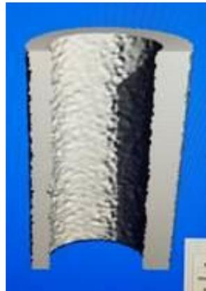
Incident Tubing: wall thickness is non-uniform (Bad)
